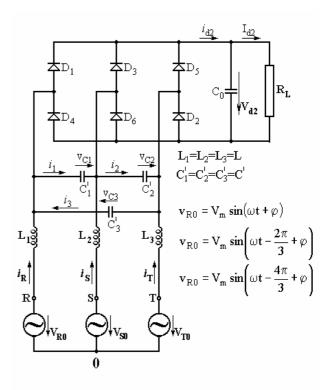
Fig.3. RNSIC converter with capacitors on the AC side
